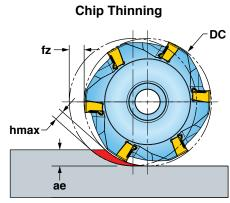
\* When ae is less than 25% DC, recommend use of Chip Thinning Calculator to ensure hmax falls within fz range.
